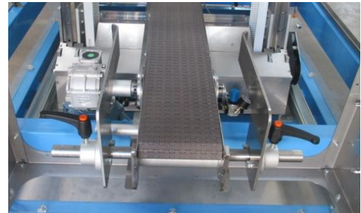
Detail of the hand-wheel adjustment of the lateral guide
