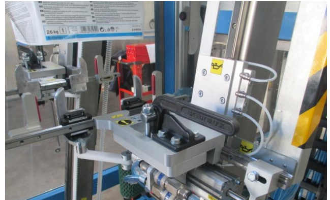
Quick format change over on the sleeve's clamps
